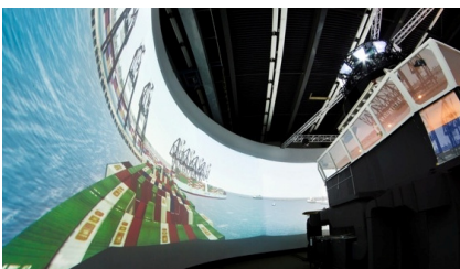
FMBI, bridge house with cylindrical projection wall
